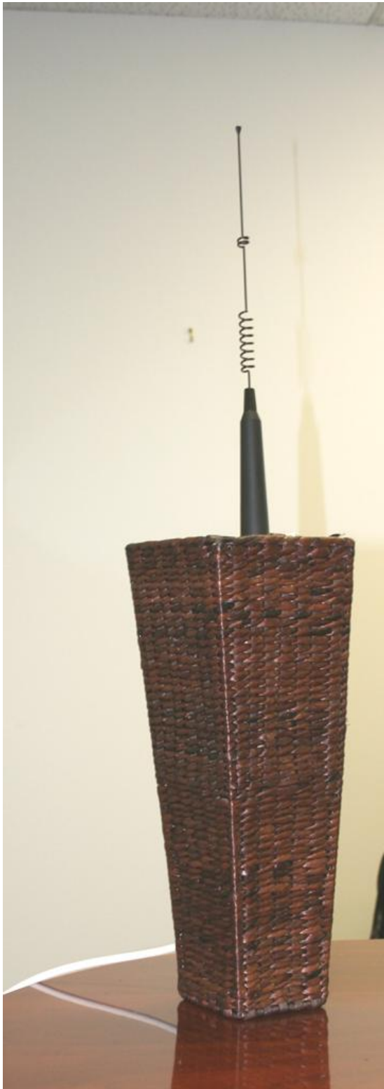
Figure 11. Antenna camouflaged inside or on a non- metallic vase which can be placed on a shelf or cabinet as high up as possible to get good coverage
